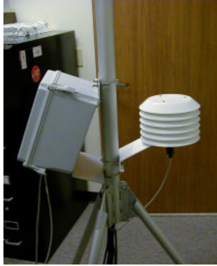
Figure 2.3 Control Unit and Temperature Sensor Assembly
